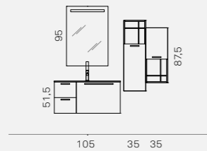
E.LY 41 (page 44-45) L 105 x P 51 cm + pensili - wall unit maniglia - handle art.323
